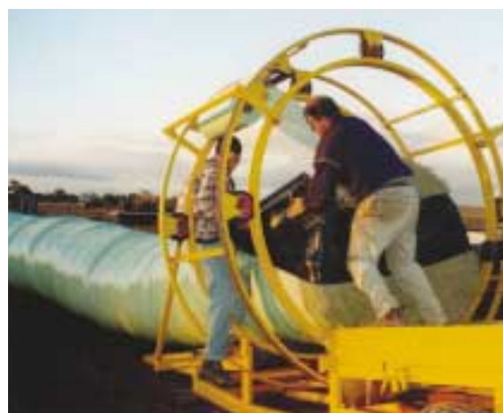
Sealing the haylage bales
