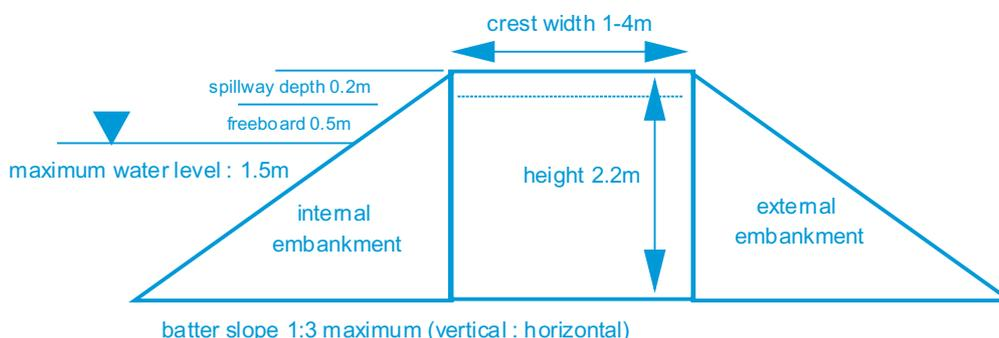
**Figure 5. Typical embankment cross section**
