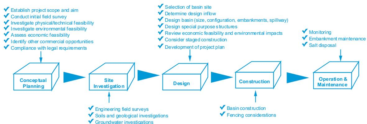
Figure 1. Process for development of an evaporation basin
