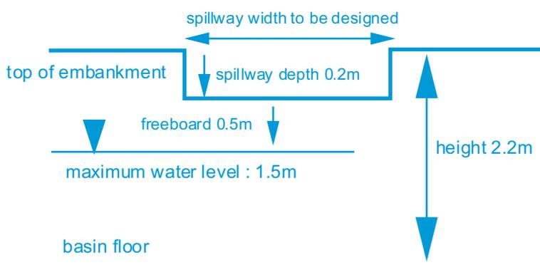
Figure 7. Cross section of spillway
