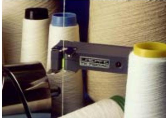
*The CSIRO Dark Fibre Detector (left) uses balanced illumination from above and below a thinly spread sample constrained between two glass plates to make objectionable fibres more visible. The SiroCLEAR™ technology (right) is an on-line optical sensing device that detects and removes contamination from undyed yarns.*
