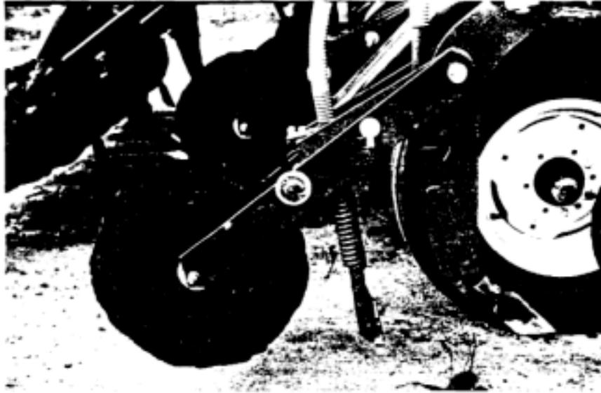
Figure 6. A second tine for shallower sowing about 15 mm to one side on Valcon Equipment Limited's Conserva-Pak® air seeder (P0 Box 417, Indian Head, Saskatchewan, Canada S4G 2K0). The press wheel also controls the depth of sowing.
