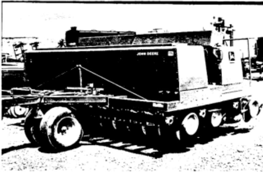
Figure 13. The John Deere 750 Series No-Till Drill is also marketed with front openers for deep placement of fertilizer nitrogen between each pair of sown rows.
