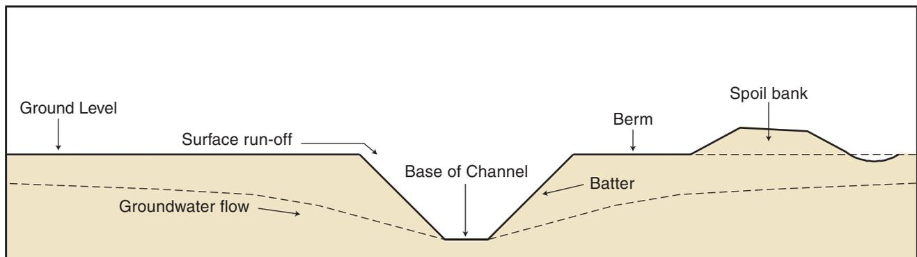
Figure 1. An open deep drain with a spoil bank or levee on one side
