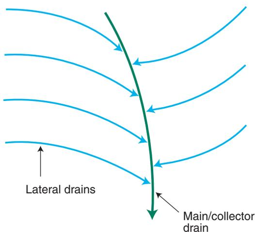
Figure 4b. Herringbone layout of drains
