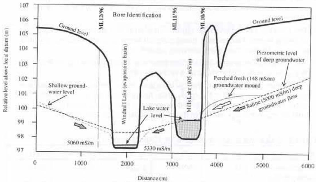
Figure 9: The Mills Lake is partly fed by a fresh groundwater mound from the east which keeps it fresh. The fresh groundwater is perching on a saline regional aquifer flowing towards Windmill Lake. Windmill Lake discharges saline groundwater over its entire area.
