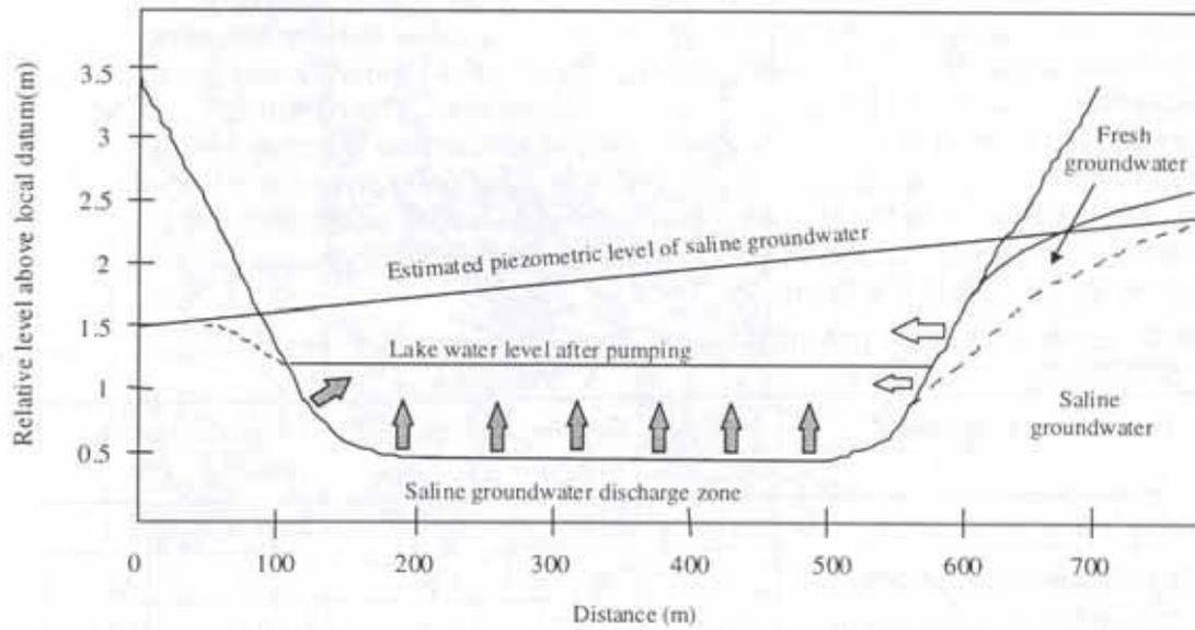
Figure 11: The situation changes when due to excessive pumping the lake's water level drops below the piezometric level of the saline aquifer. Then saline groundwater discharges into the lake and the Lake's water becomes saline.
