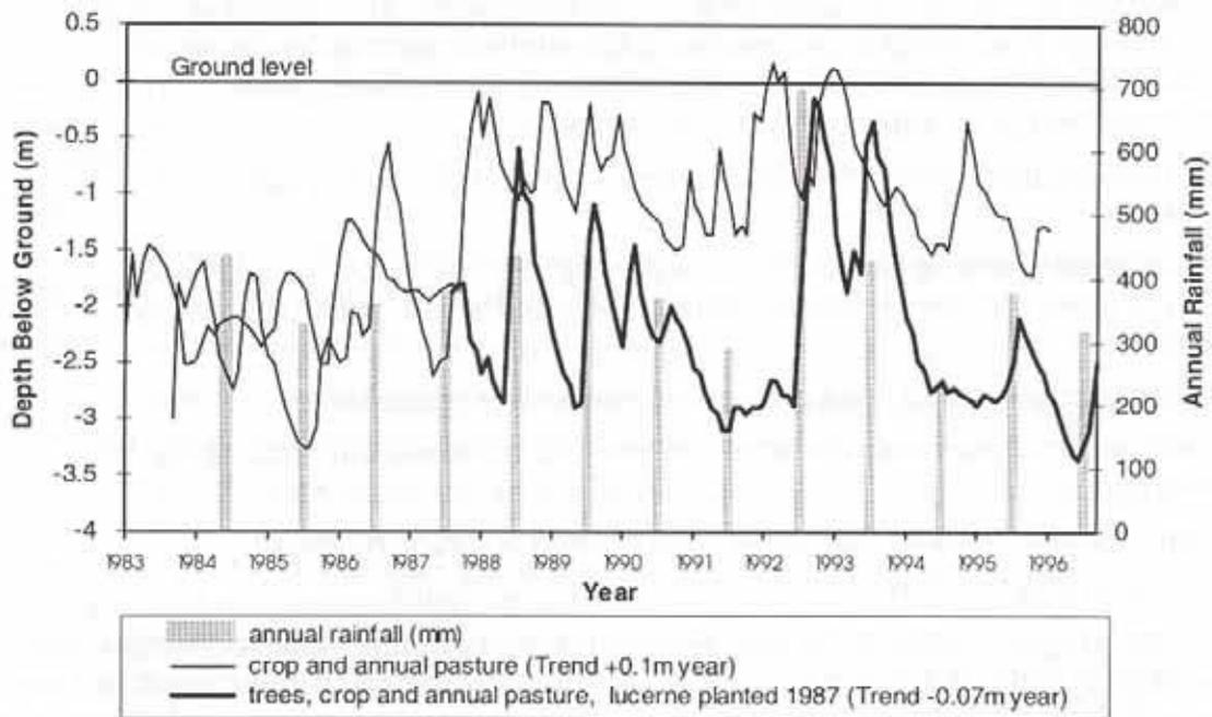
Figure 14: In Ancient Drainage Valleys, a lucerne and alley farming system has lowered groundwater levels by 1.7 m in comparison with the traditional crop and annual pastures rotation.
