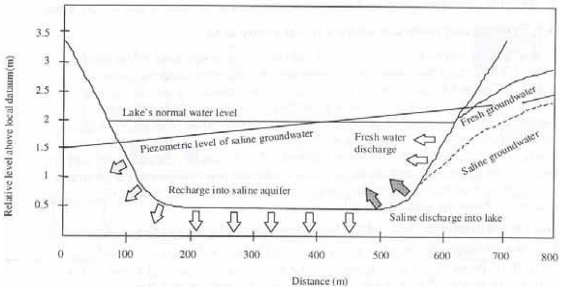
Figure 10: At high water levels, the Mills Lake receives a large discharge of fresh water and a small amount of saline groundwater. The pressure is such that the Lake's water recharges the saline aquifer on the western side. In this situation, the Lake's water remains reasonably fresh.
