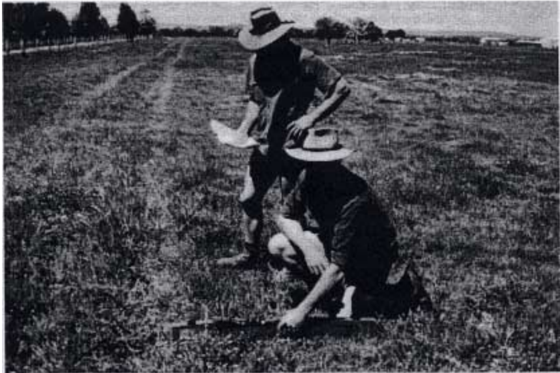
Figure 1. The EM38 being used during a transect survey at Waterloo. It is easy if one person takes the readings and the other records them in a notebook.
