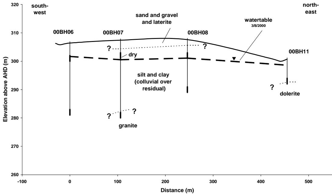
Figure 2-3. South-west to north-east cross-section from bores 00BH06 to 00BH11 (see Figure 2-1 for location)
