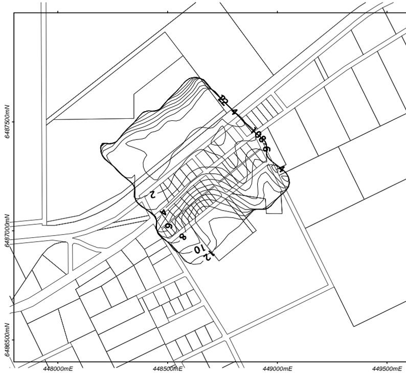
Figure 3-2. Depth to groundwater (in metres, contour intervals are 1 m) for steady-state simulation
