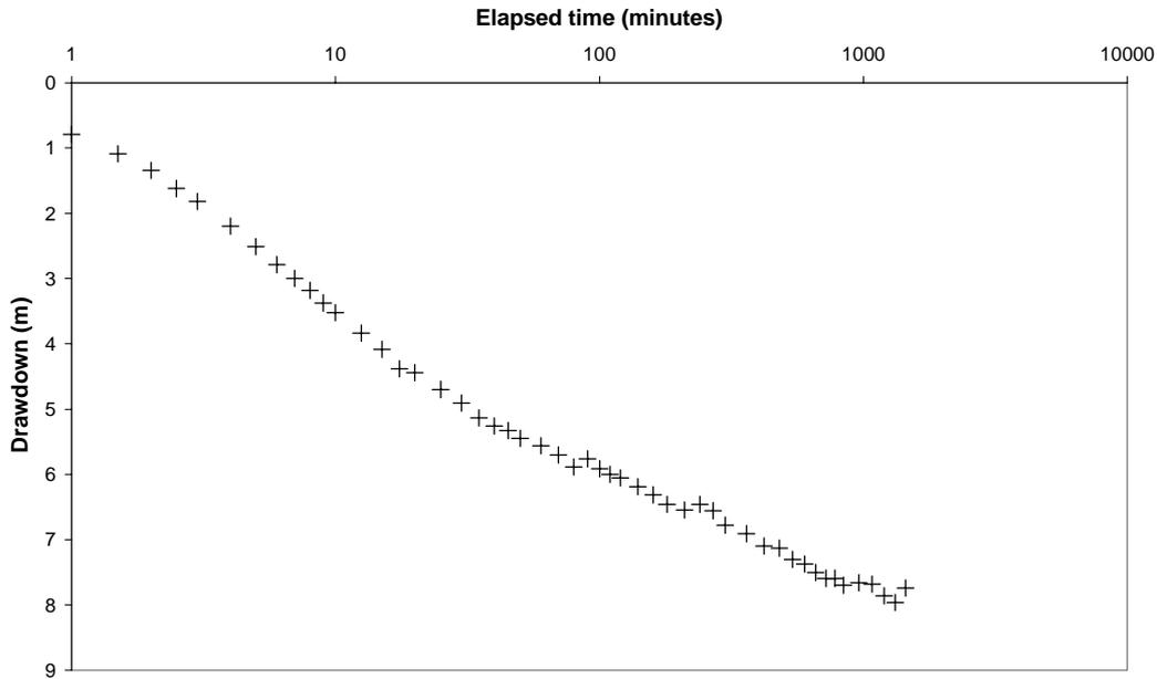
Figure 2-6. Production bore drawdown versus time for constant rate test
