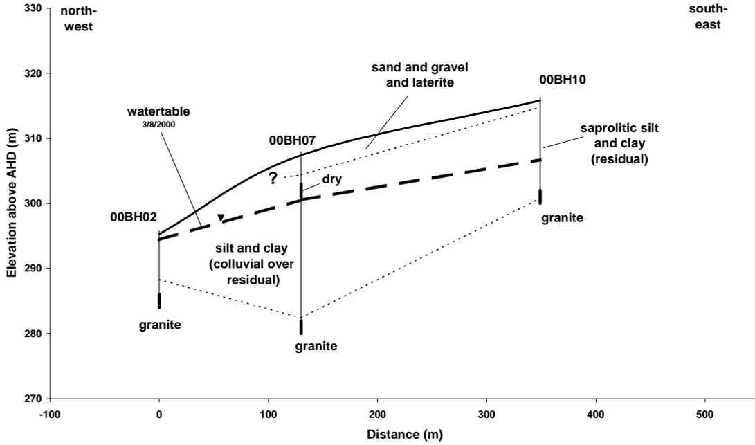
Figure 2-4. North-west to south-east cross-section from bores 00BH02 to 00BH10 (see Figure 2-1 for location)
