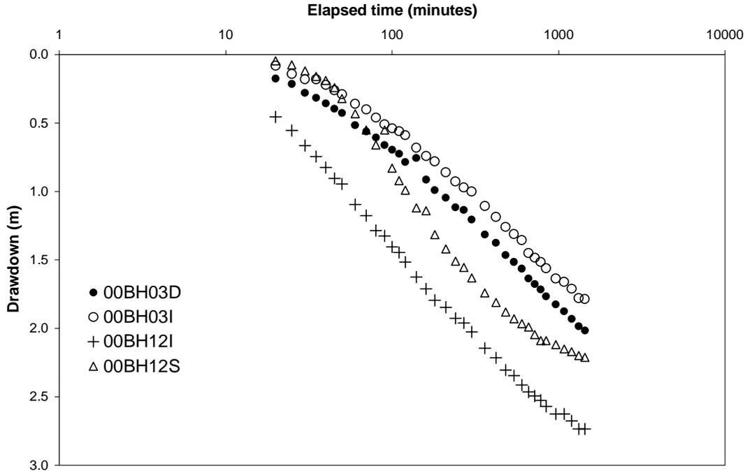
Figure 2-7. Monitoring piezometer drawdowns versus time for constant rate test (piezometers were about 15 m away from the production bore)
