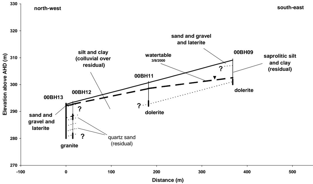
Figure 2-5. North-west to south-east cross-section from bores 00BH13 to 00BH09 (see Figure 2-1 for location)
