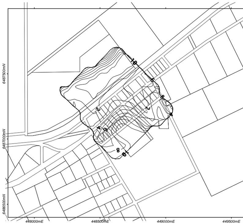
Figure 3-7. Depth to groundwater after 30 years (in metres, contour intervals are 1 m) for drainage simulation
