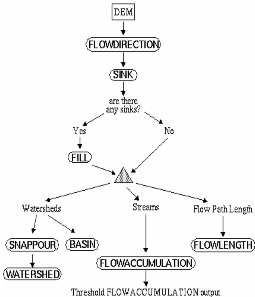
Figure 2. The process of extracting hydrologic information from a DEM
