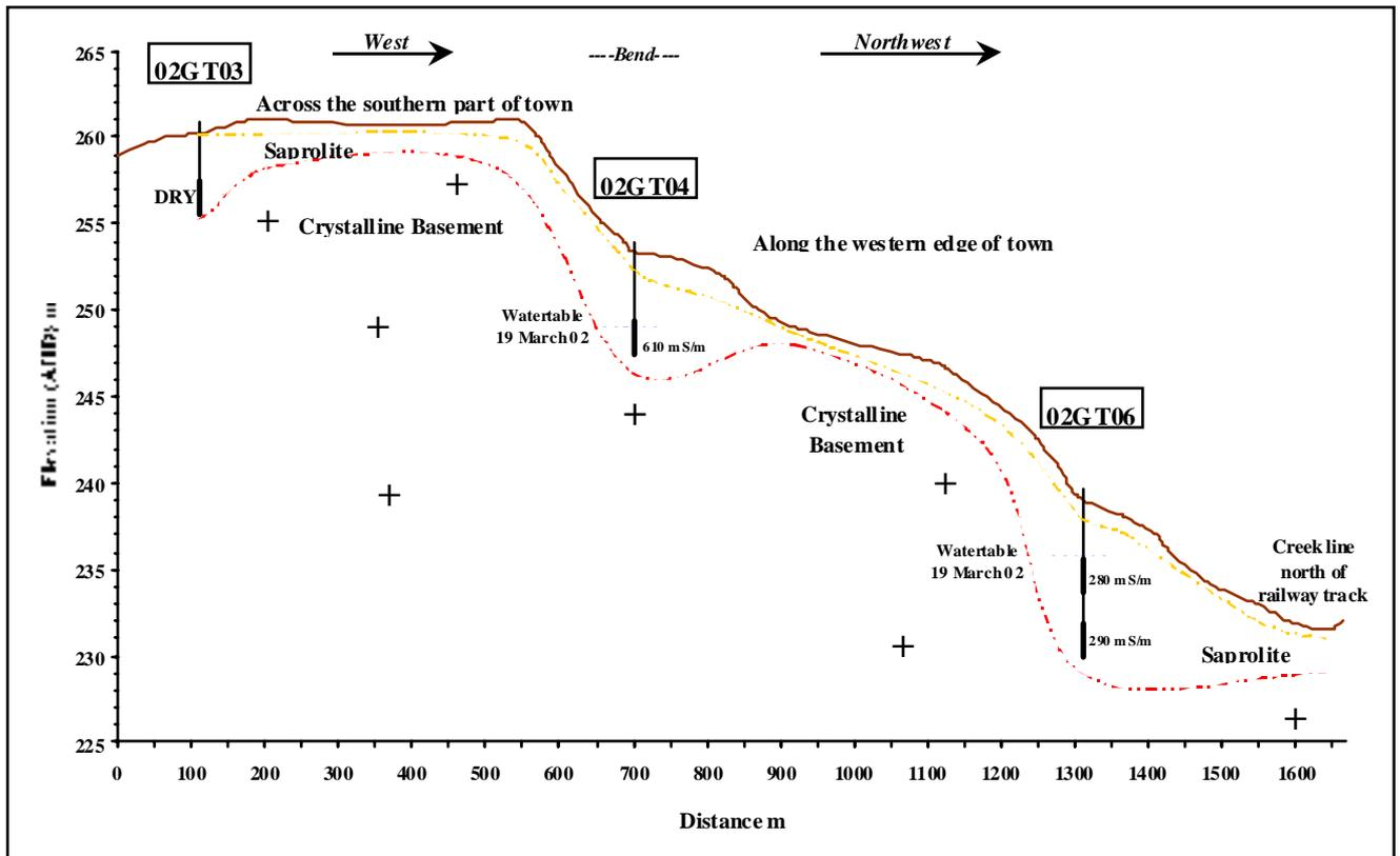
Figure 2-1: Cross-section constructed from drilling results and conceptual model of profile
