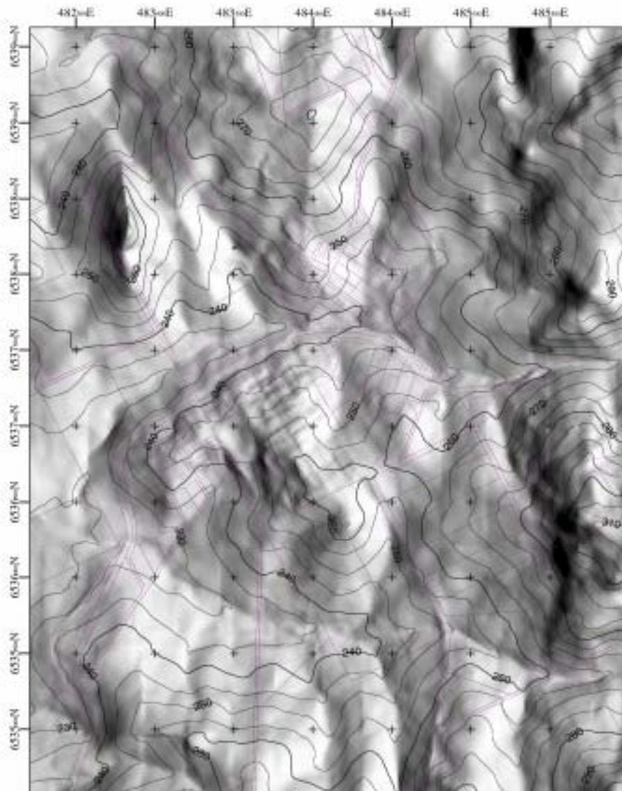
Figure 1-2. Shade-enhanced image of DEM (sun angle: azimuth =  $82^{\circ}$ , elevation =  $56^{\circ}$ ) with surface elevation contours (Australian Height Datum) at 5-metre intervals and some cadastral information. Goomalling is located on the hill in the centre.
