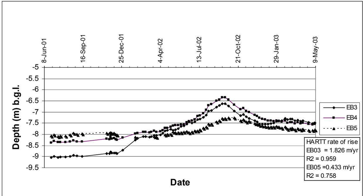
Figure 5.4. Monitoring bore water level response to inflows to the evaporation basin - northern side
