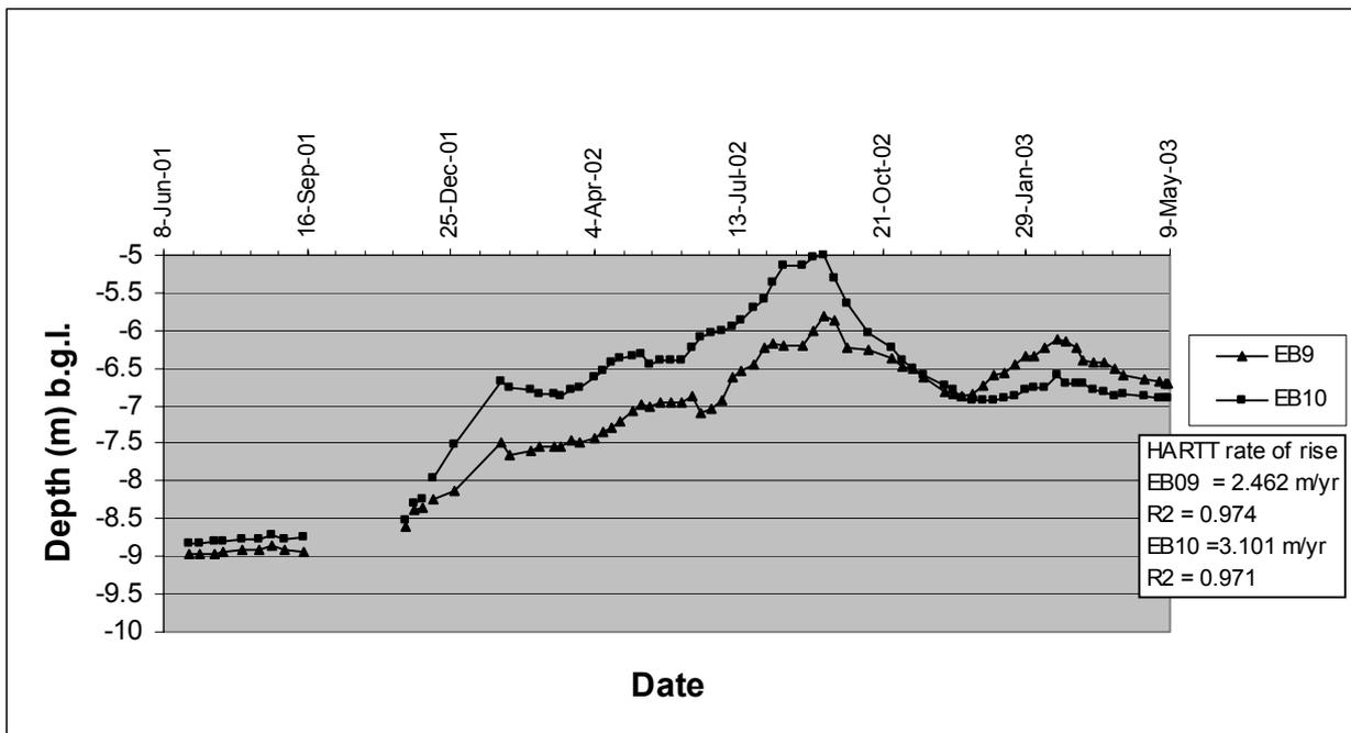
Figure 5.7. Monitoring bore water level response to inflows to evaporation basin - away from the influence of evaporation basin
