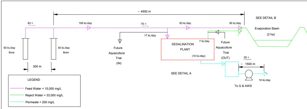
Figure 3.2. Diagram of daily groundwater distribution
