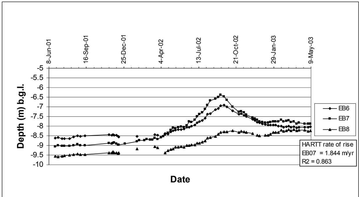
Figure 5.5. Monitoring bore water level response to inflows to the evaporation basin - southern side
