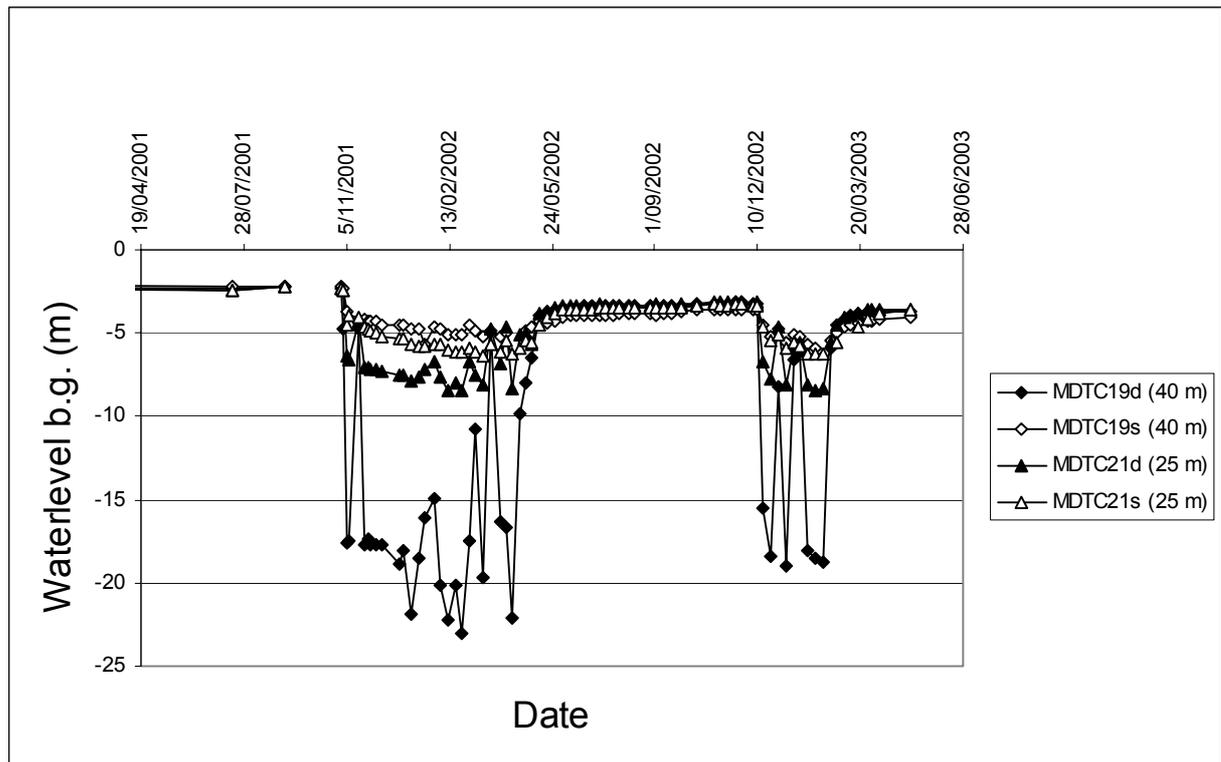
Figure 3.8. Deep and shallow aquifer water level response to pumping at PB1
