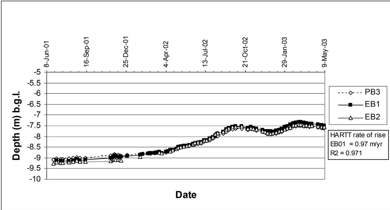
Figure 5.2. Monitoring bore water level response to inflows to evaporation basin, western side
