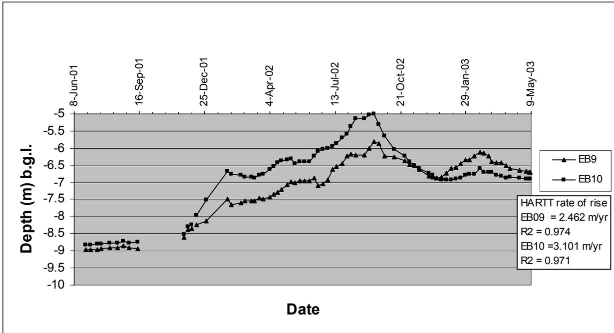
Figure 5.6. Monitoring bore water level response to inflows to evaporation basin - below basin
