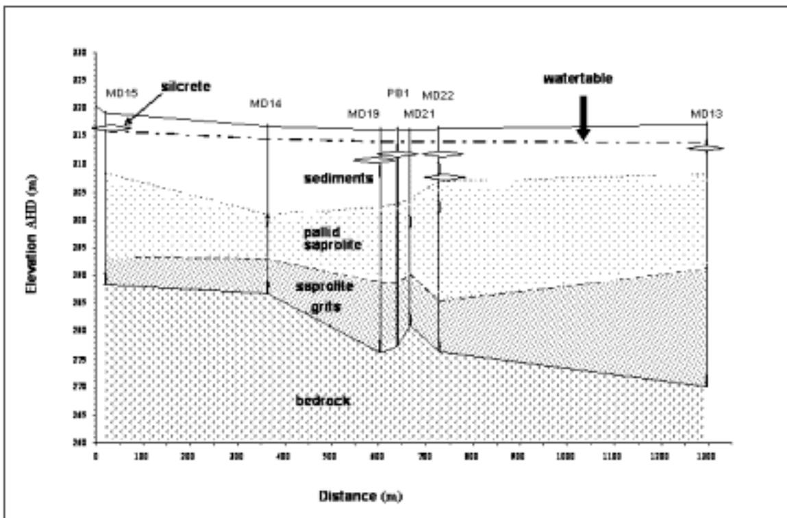
Figure 3.4. North-south hydrogeologic cross-section of Merredin town
