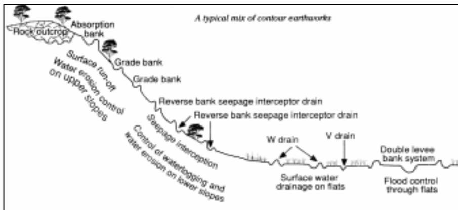
Figure 11. Schematic representation of some typical surface earthworks (after, Negus unpub & Lefroy n.d.)
