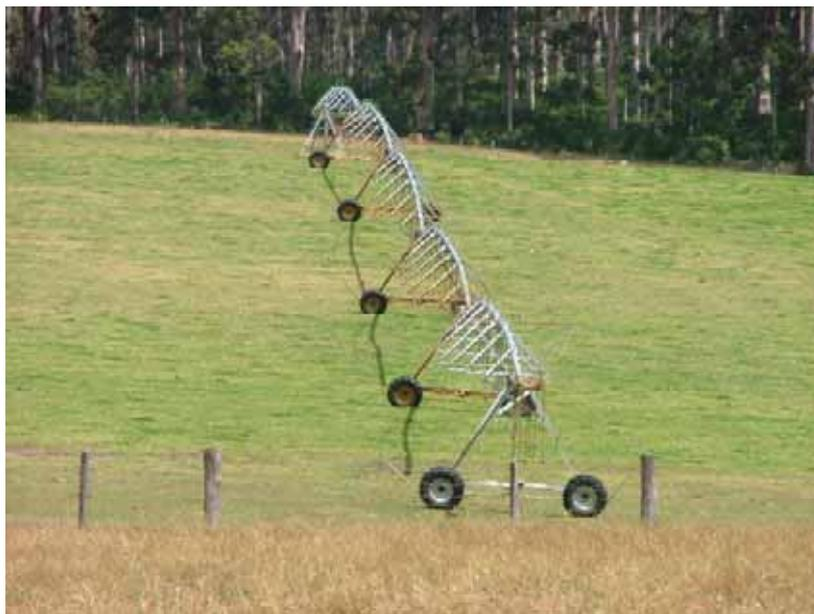
*Centre pivot used to irrigate and spread effluent*
